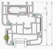
Linktrusion® continuous Glass Fibre Reinforced Strips
